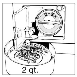
Turn the lint trap lid counterclockwise 2 - 3 times. Do **not** remove it. Approx. 2 quarts of water will drain out of the hose.
